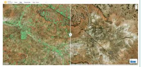
*Note*: A screenshot of the Restoration Mapper prototype, which displays detailed, wall-to-wall maps of the spatial distributions of trees with canopy diameters larger than 2 m. The maps are created using artificial intelligence algorithms and freely available 10-m-resolution satellite data (Sentinel 2). The image on the left shows the pixels of tree cover, and that on the right shows the raw satellite imagery. *Source:* Brandt and Stolle (in prep.).
